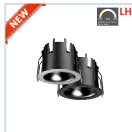
HLR-2624 (5W) Size : Ø63mmx52mm Cut-Out : Ø55mm Housing Colour : Black Ring Available : White+Black / Black+Black Reflector Available : Gun Black
