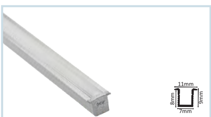
HLL-1050: CONCEALED BODY - FULL SET STANDARD LENGTH : 2MTR SIZE : 11xD9mm / CUT-OUT : 7xD8mm
